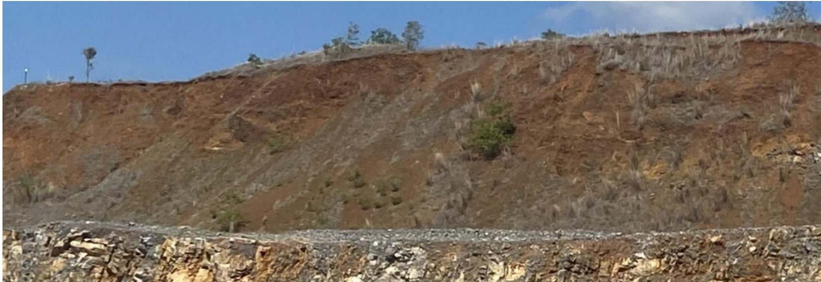
Figure 7. Bouldery clay overlying limestone on the (a) east wall and (b) north wall of Pit 4.
