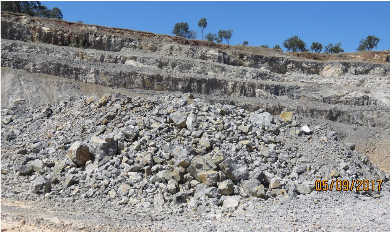
Figure A5.1. Typical muckpile highlighting the range of rock shapes and sizes generally exposed on the benches. The sizes and shapes generated in the simulation are consistent with these observations.
